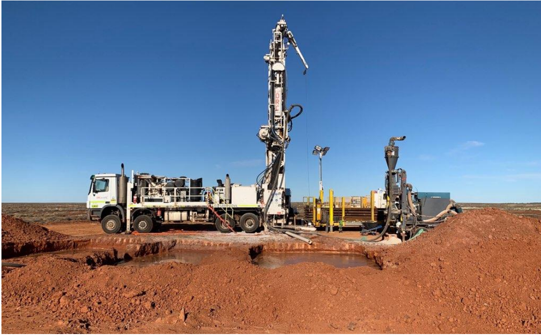
Figure 1: DRC Drilling – drill rig and support equipment set up on HWDD_02 at Horse Well prospect.
